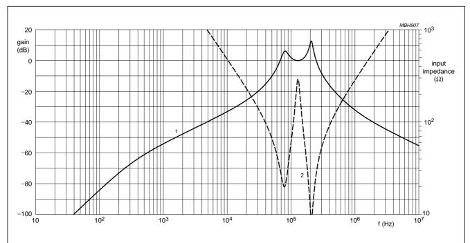
Main features of the coupling network: 50 Hz rejection >80 dB; anti-aliasing for the digital filter >50 dB at the sampling frequency ( $^{1}\!\!/_{2}f_{osc}$ ). Input impedance always higher than 10  $\Omega$  within the 95 to 148.5 kHz band.
